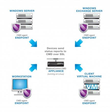
Each CMD EndPoint reports to the CMD appliance using SSL over Port 443.
